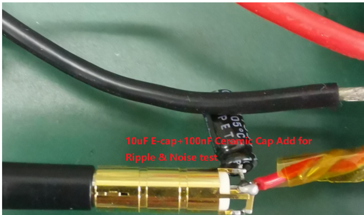
Figure 7. Ripple and noise test setup probe: 10 \mu electrolytic capacitor and 100 nF ceramic capacitor added
