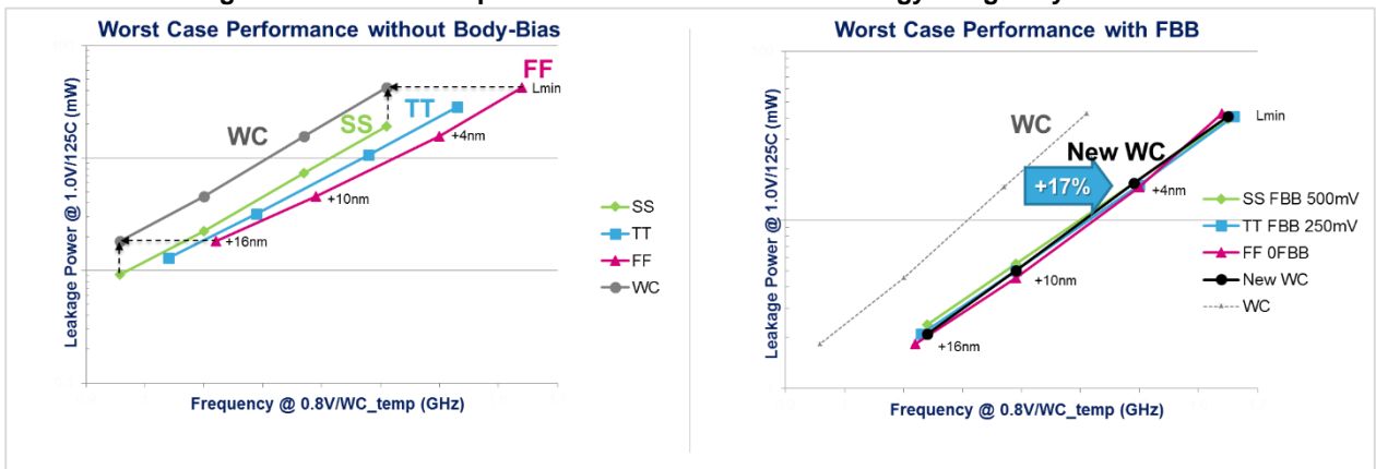
Figure 22: Process compensation in 28nm FD-SOI technology using body-bias
