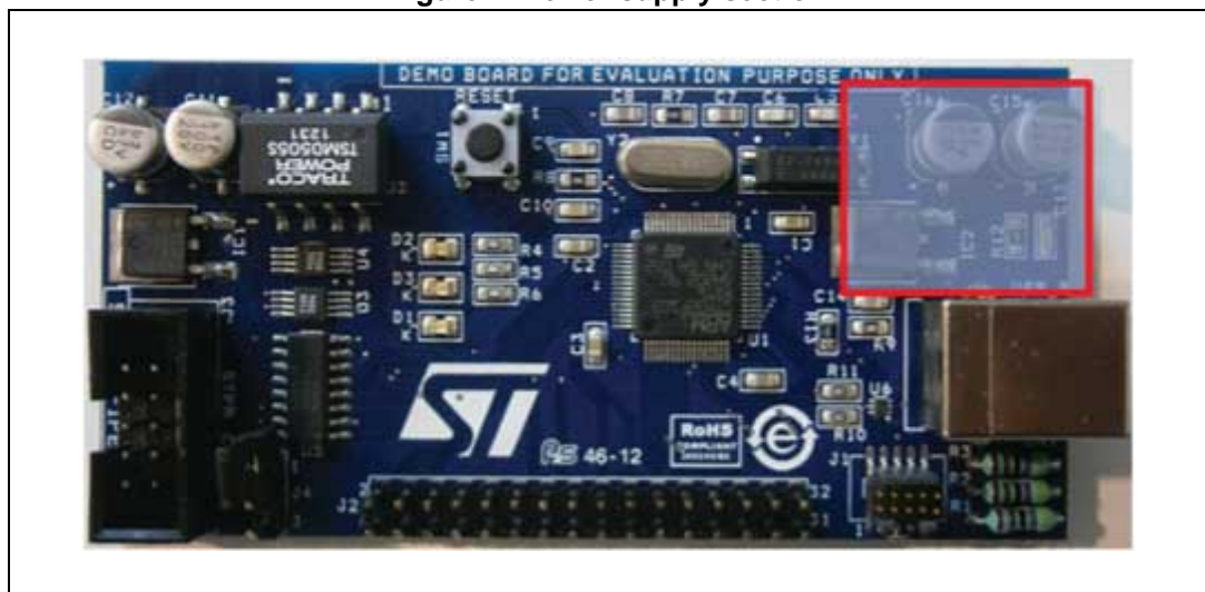
Figure 4. Power supply section
