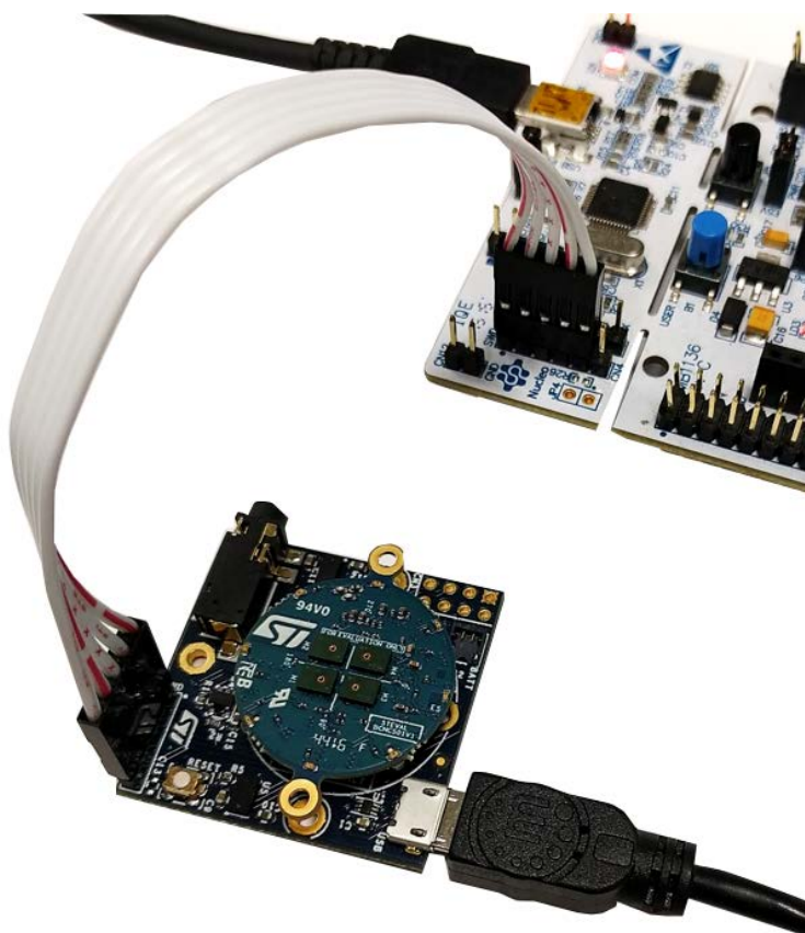
Figure 19. SWD connections with 5-pin flat cable
