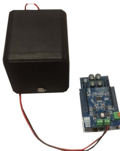
Figure 11. Loudspeaker connected to the board stack
