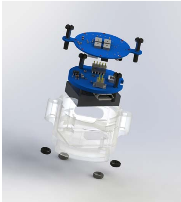
Figure 13. BlueCoin, cradle and plastic case: assembled
