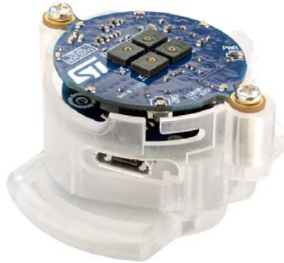
Figure 13. BlueCoin, cradle and plastic case: assembled
