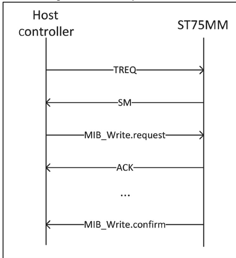
The MIB\_Read request coming from the host controller follows the same mechanism as the MIB\_Write.
