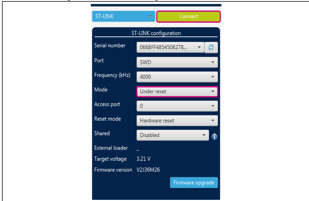
Figure 19. STM32CubeProgrammer connection menu
