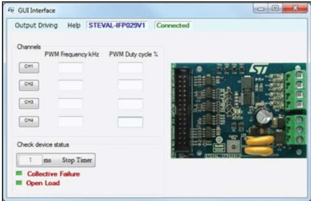
Figure 9: GUI interface (collective failure/open load)
