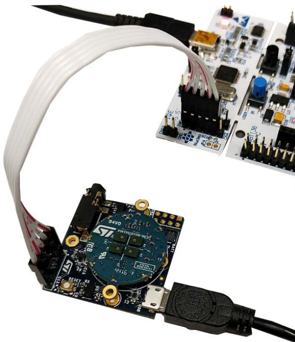
Figure 35. BlueCoin-STM32Nucleo: SWD connections with 5-pin flat cable
