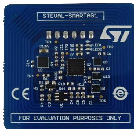
Figure 22. STEVAL-SMARTAG1 evaluation board
