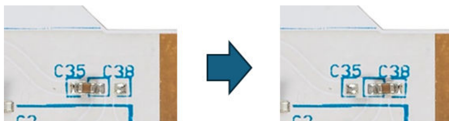
Figure 25. Modification for SMA path (MB1355C-02)
