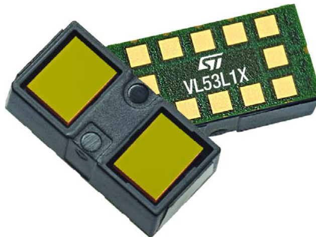
Figure 1. VL53L1X sensor module
