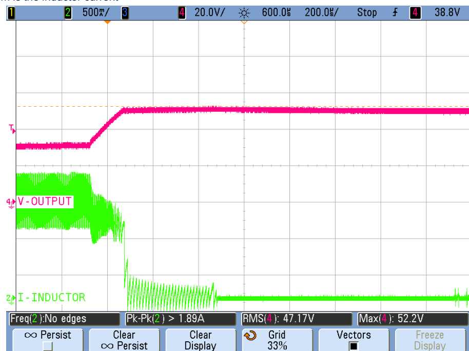
Figure 18. Open circuit protection behavior
