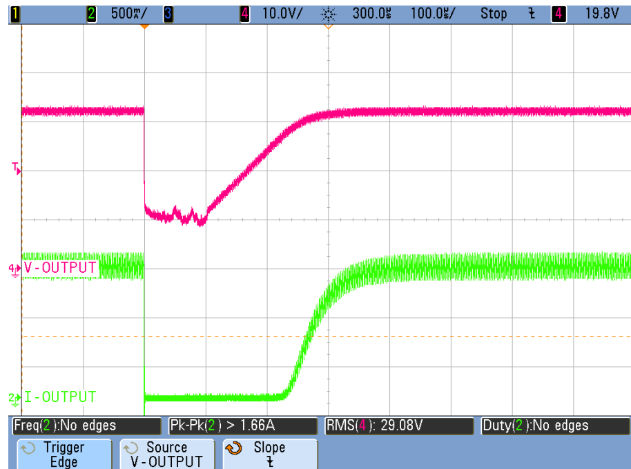
Figure 18. Open circuit protection behavior
