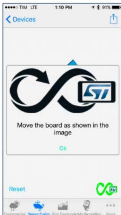
Figure 20. STBLESensor Compass and Level app - starting the calibration
