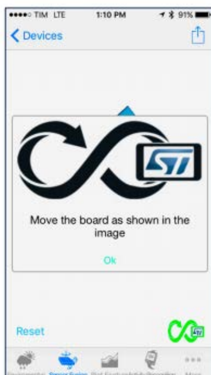
Figure 34. Sensor fusion app - enabling magnetometer calibration
