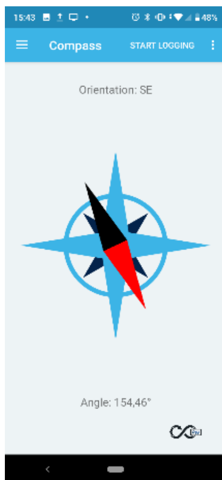
Figure 21. STBLESensor Compass and Level app - orientation screen
