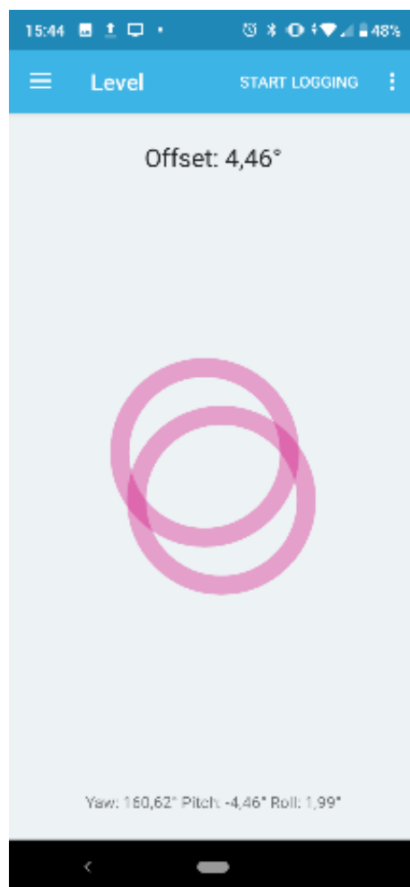
Figure 22. STBLESensor Compass and Level app - offset example 1
