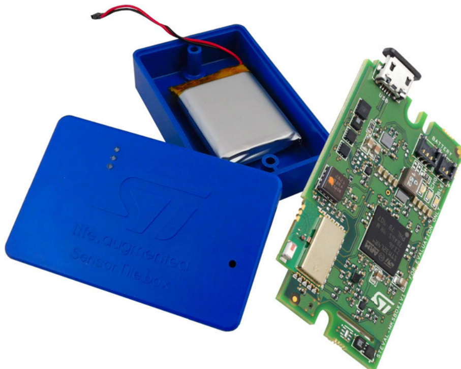
Figure 1. STEVAL-MKSBOX1V1 (SensorTile.box) multi-sensor development kit
