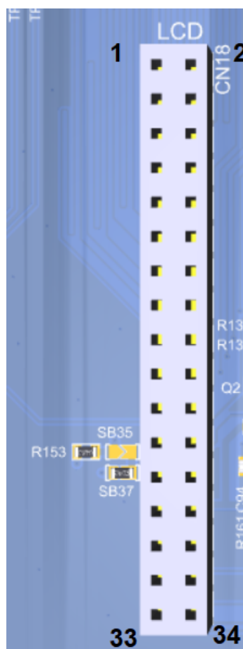
Figure 27. CN18 LCD connector pinout
