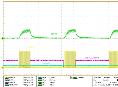
Figure 22. EVAL-IBD002-35W VDIMM = 0.5 V
