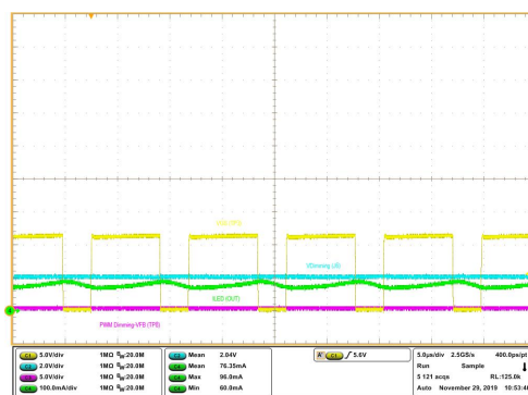
Figure 17. EVAL-IBD002-35W VDIMM = 2 V
