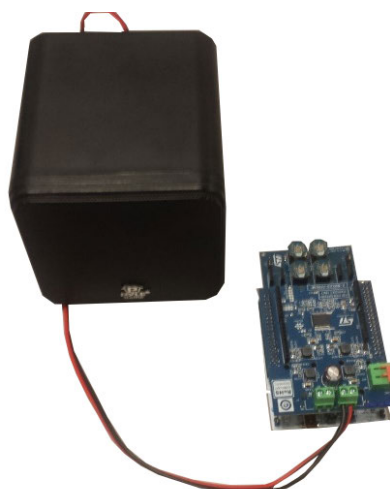
Figure 7. Loudspeaker connected to the board stack
