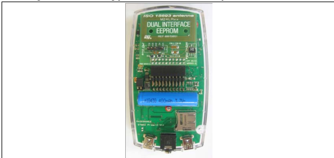
Figure 50. Connecting your reference antenna to your STM32-PRIMER2
