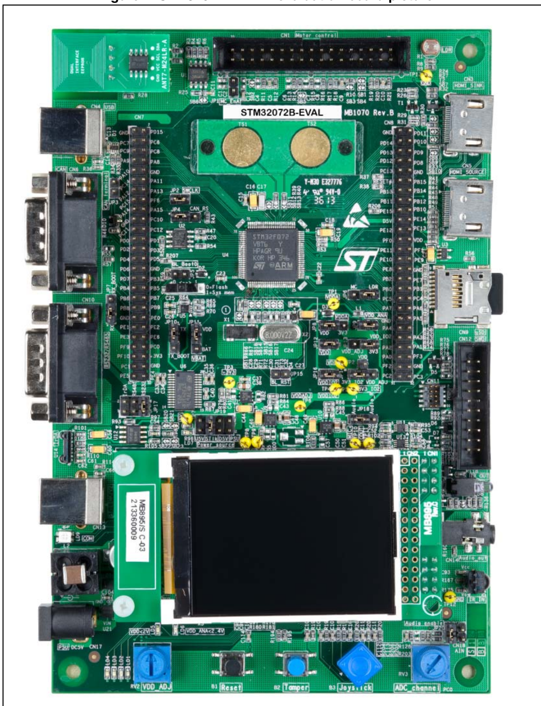
Figure 1. STM32072B-EVAL evaluation board picture (1)
