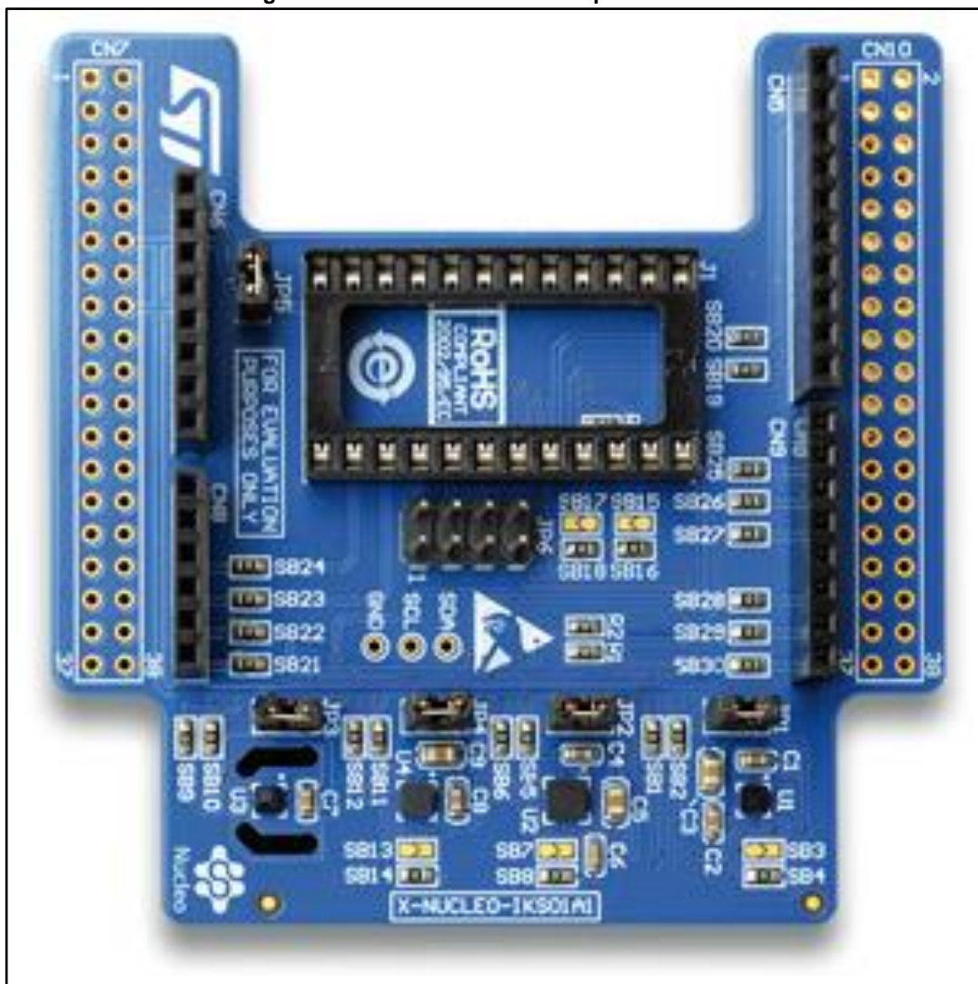
Figure 33: X-NUCLEO-IKS01A1 expansion board
