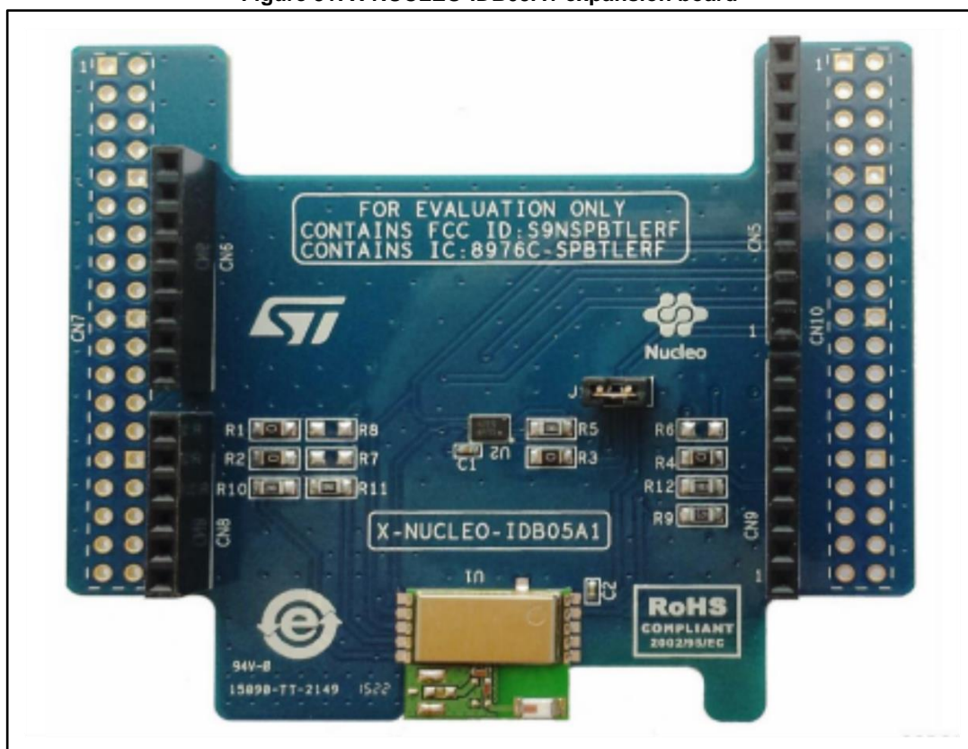
Figure 31: X-NUCLEO-IDB05A1 expansion board
