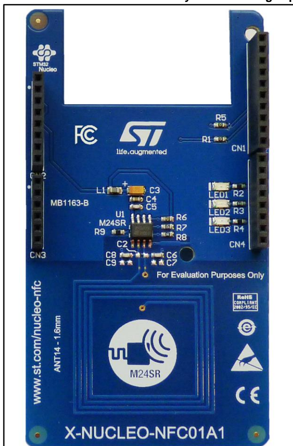
Figure 32: X-NUCLEO-NFC01A1 M24SR64-Y dynamic NFC tag expansion board
