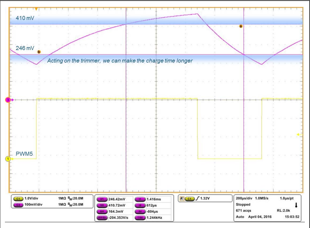
Figure 15. PWM5 and output voltage regulation - oscilloscope plot - long charge time
