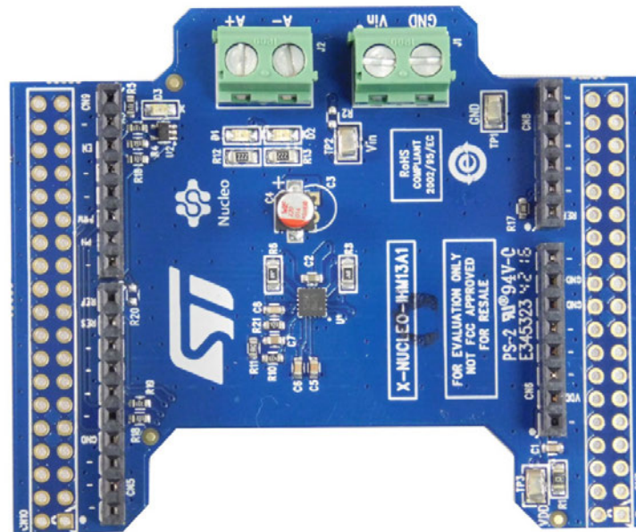
Figure 3. X-NUCLEO-IHM13A1 expansion board for STM32 Nucleo
