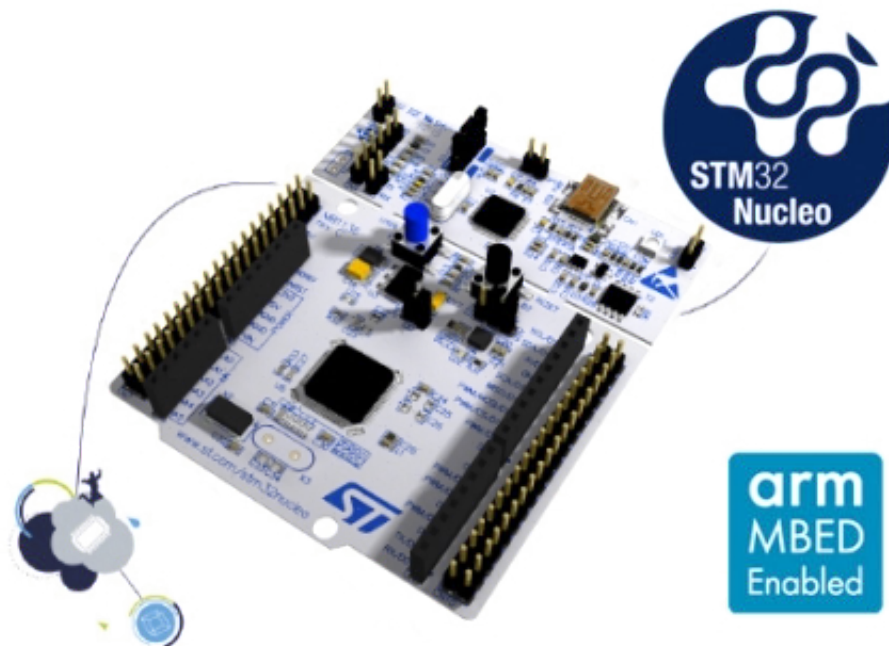
Figure 2. STM32 Nucleo board
