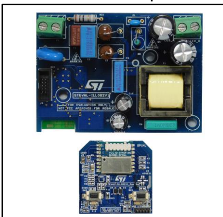
Figure 2: STEVAL-ILL082V1 evaluation board plus remote controller (bottom view)
