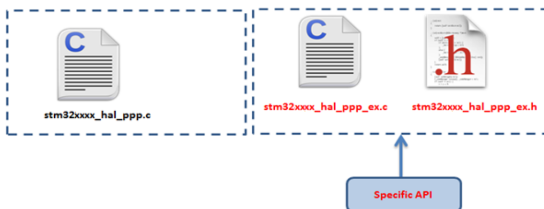
Figure 2. Adding device-specific functions
