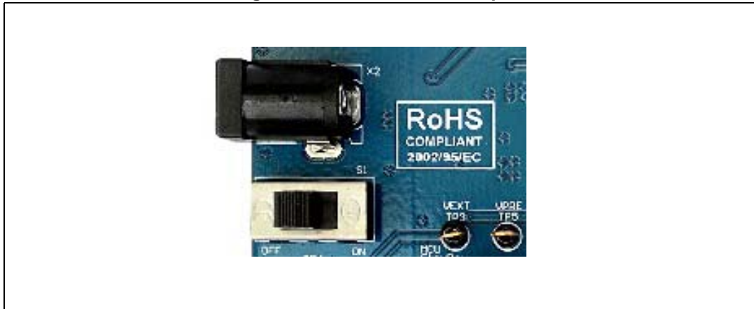
Figure 2. PSU section - DC input
