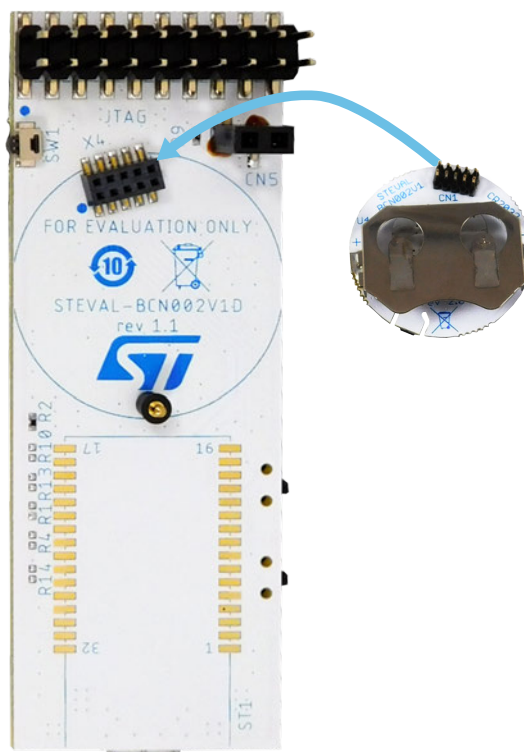
Figure 10. Connectors to mount the sensor node on the host board
