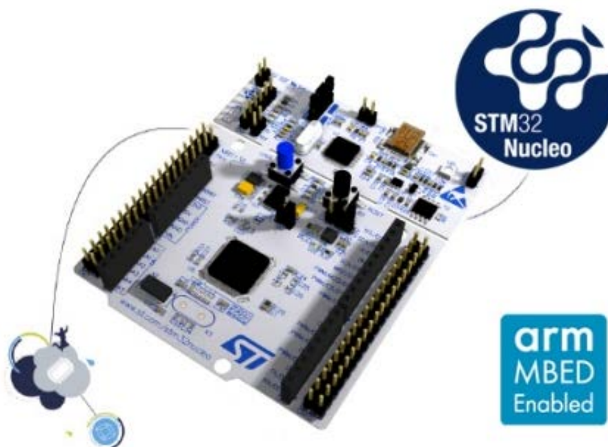
Figure 11. STM32 Nucleo board
