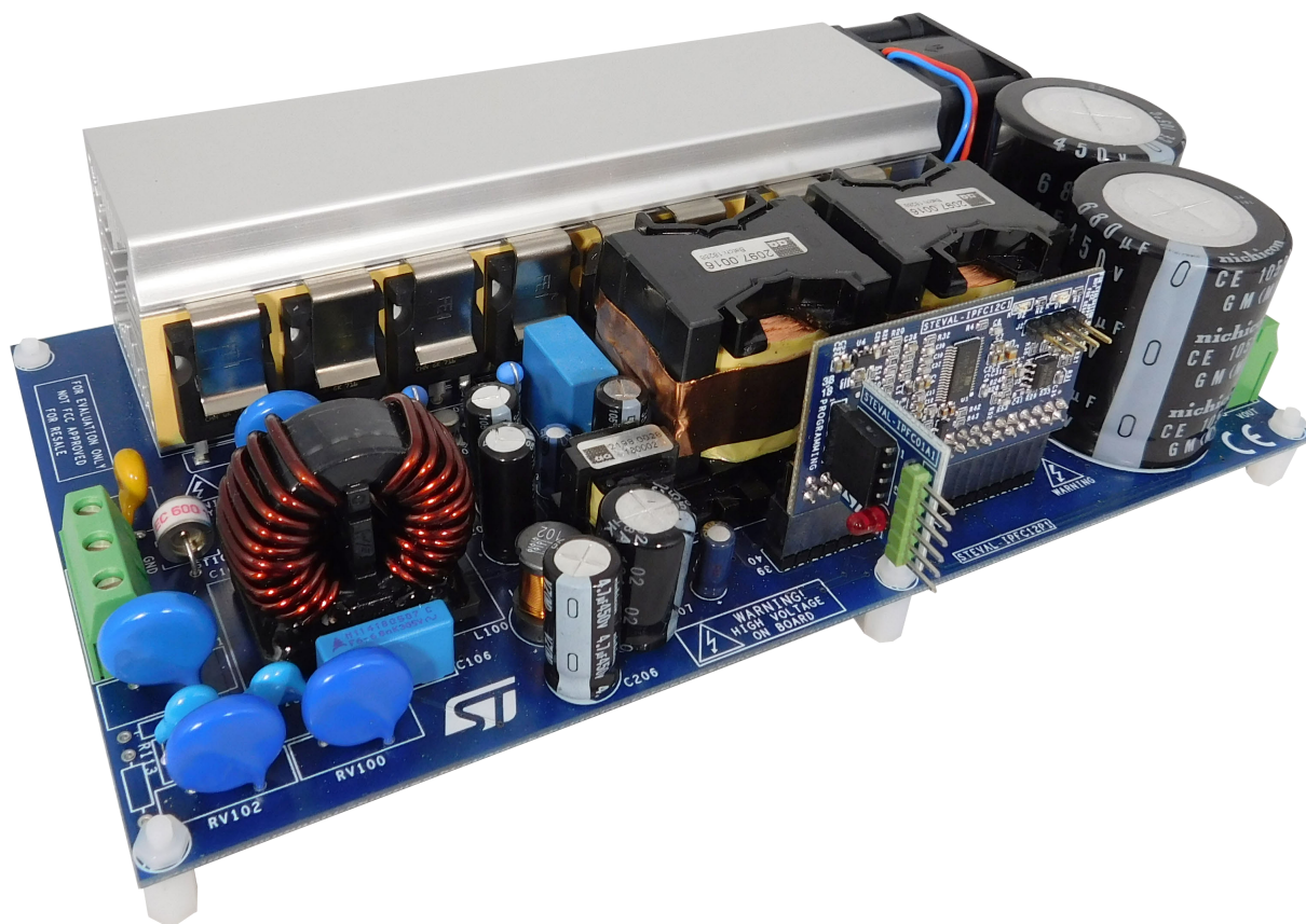
Figure 1. STEVAL-IPFC12V1 evaluation kit with power, control and adapter boards
