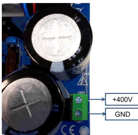
Figure 4. STEVAL-IPFC12P1 DC output connection
