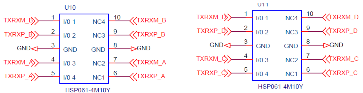
Figure 4. 1 Gb/s Ethernet ESD protection schema
