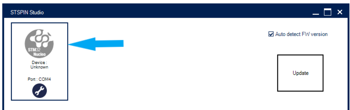
Figure 2. Connection window - no communication with the board
