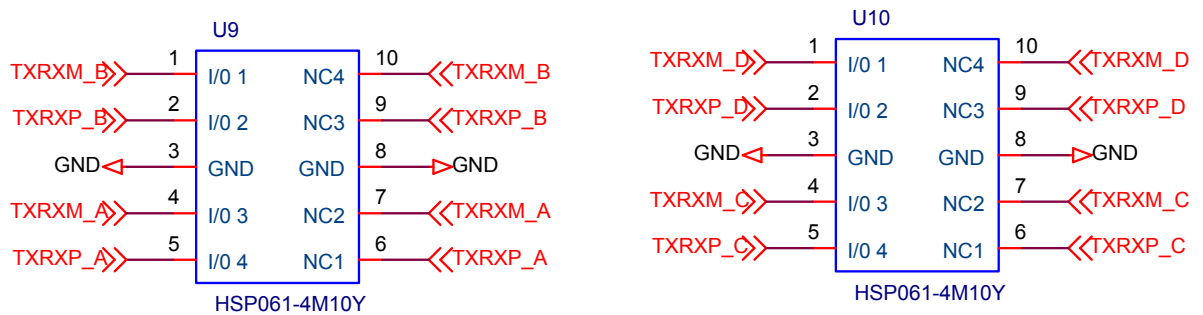
Figure 4. 1 Gb/s Ethernet ESD protection schema
