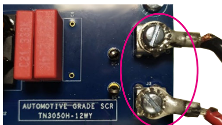
Figure 9. STEVAL-DPSTPFC1 output HVDC connection
