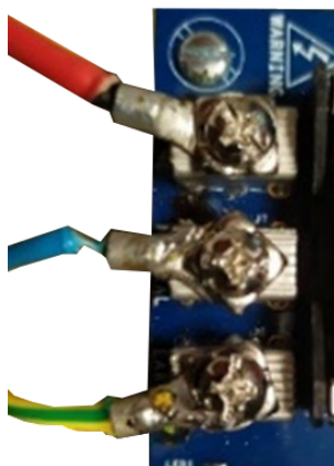
Figure 8. AC line wire connection overview
