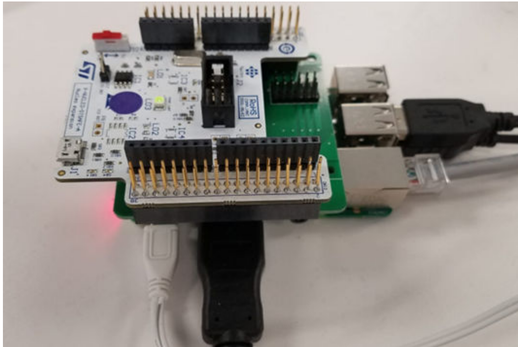
Figure 7. STSAFE-A1xx expansion board on an RPi board using jumper wires
