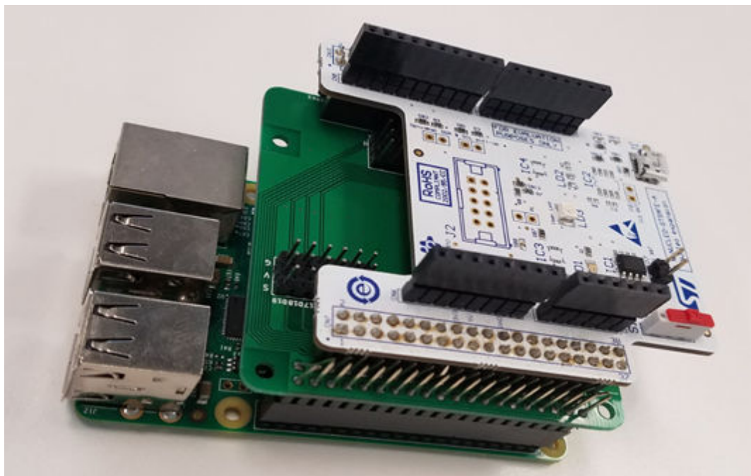
Figure 5. Example with the STSAFE-A1xx expansion board on an RPi board using the ARDUINO shield
