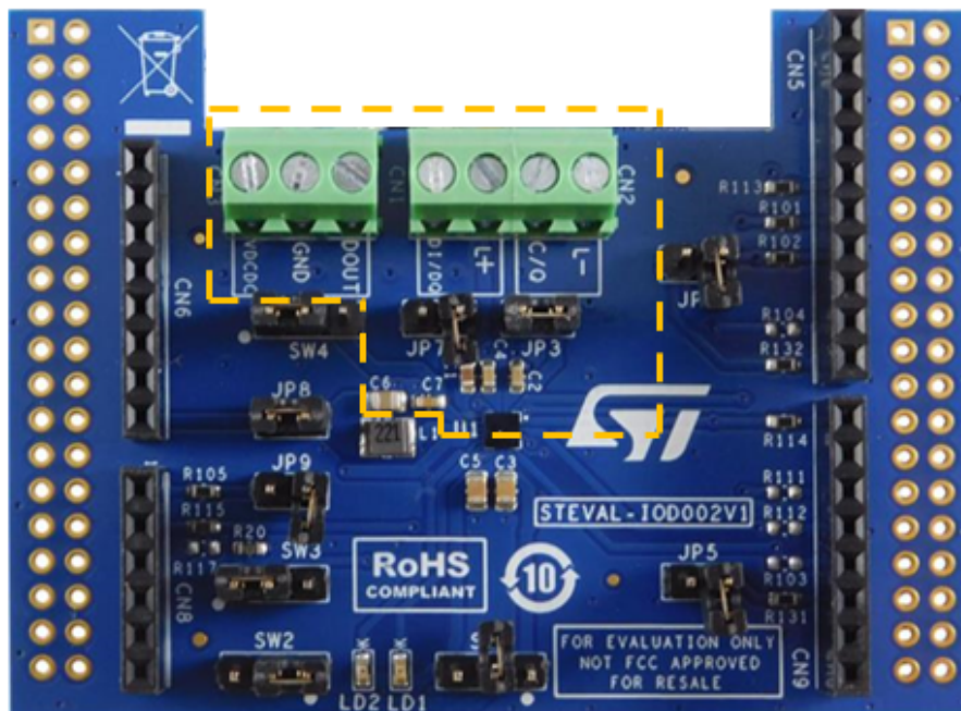
Figure 3. STEVAL-IOD002V1 expansion board power section
