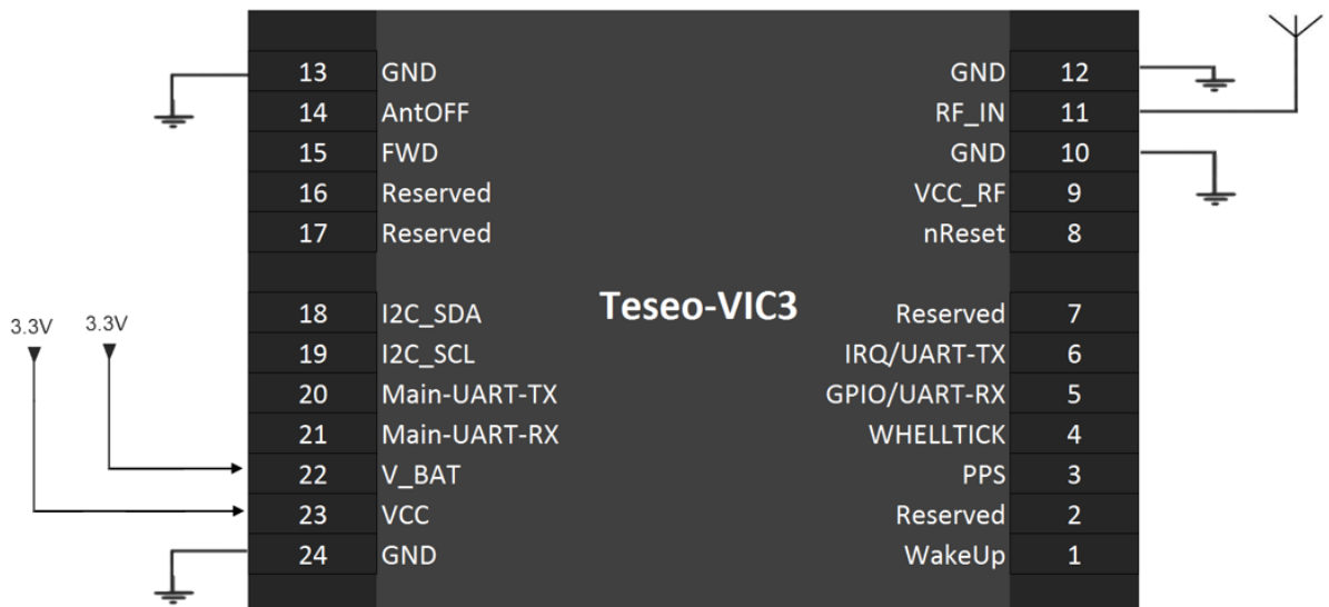
Figure 2. Teseo-VIC3 minimum connection
