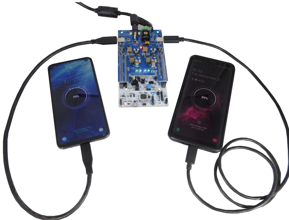
Figure 19. STEVAL-2STPD01 evaluation kit connection example - charging two mobile phones
