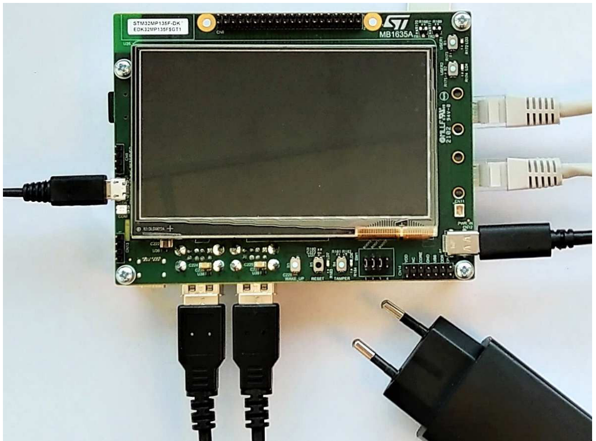
Figure 2. STM32MP135F-DK Discovery kit connections
