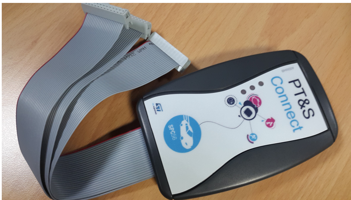
Figure 16. PT&S Connect Micro board
