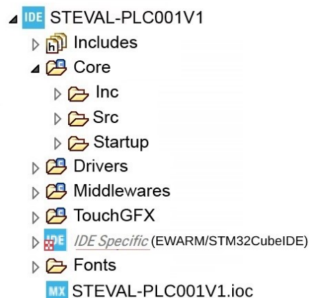
Figure 2. STSW-PLC001 folder structure
