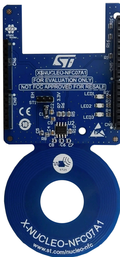
Figure 4. X-NUCLEO-NFC07A1 expansion board
