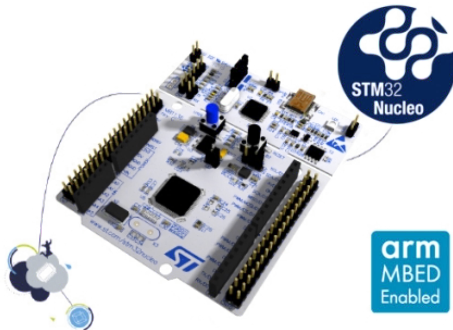
Figure 3. STM32 Nucleo board
