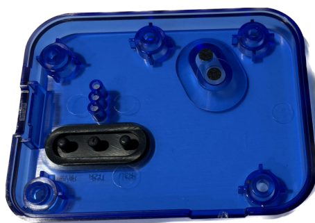
Figure 31. Vents installed on acoustic holes (inside view)
