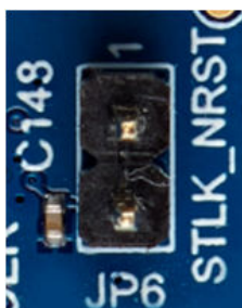
Figure 14. STLK_Nrst default configuration (JP6)
