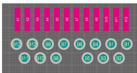
Figure 26. USB Type-C® top layer footprint pinout (CN4)
