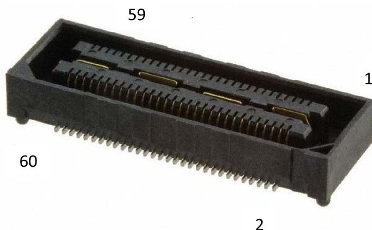
Figure 31. DSI_V3 display connector (CN2)
