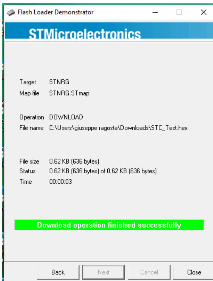
Figure 10. ST Flash Loader – STNRG programming complete
