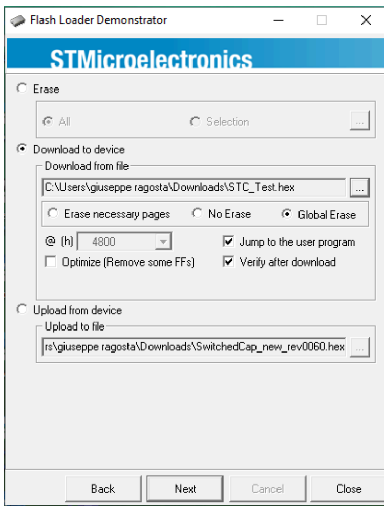
Figure 9. ST Flash Loader – STNRG programming settings
