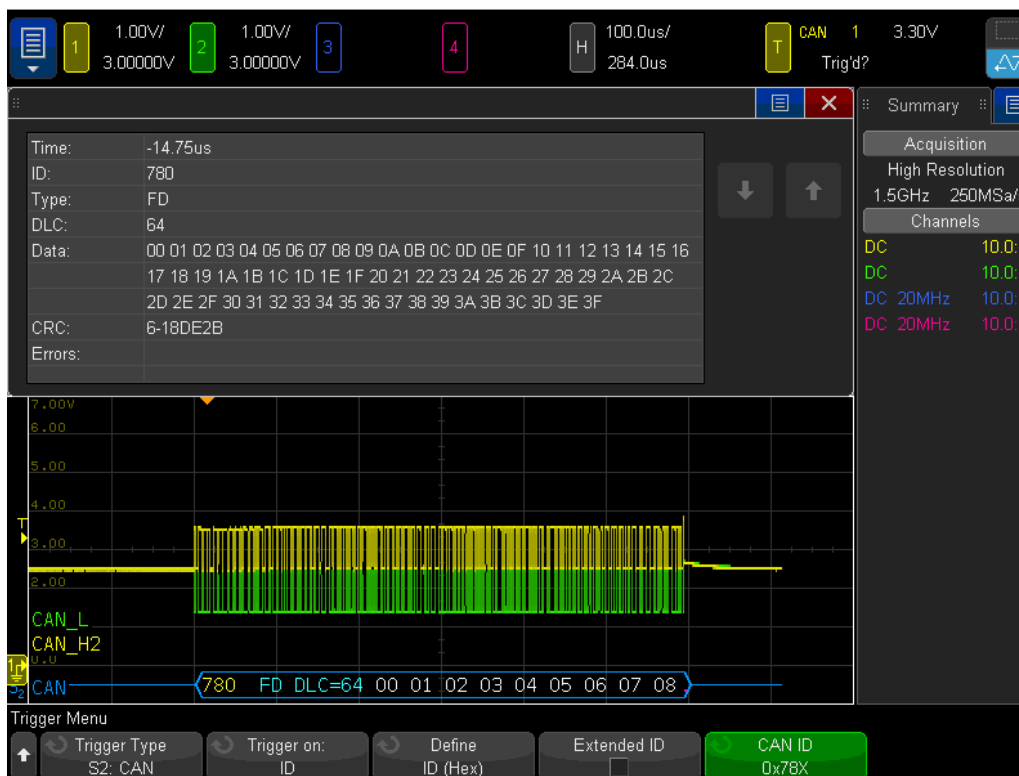
Figure 44. Broadcast PWM data send to ChainID=0 (test case 1)
