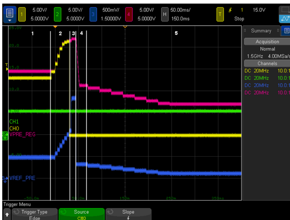
Figure 107. VREF_PRE_REG - operating example closed loop algorithm in open load
