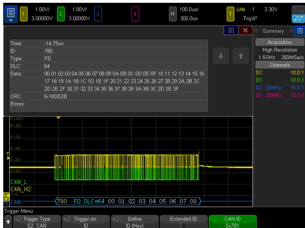
Figure 50. Broadcast PWM data send to ChainID=0 (test case 2)
