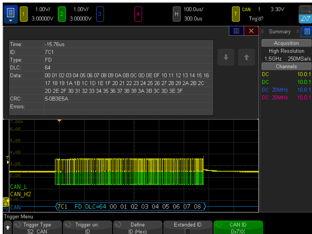
Figure 56. Broadcast current data send to ChainID=1 (test case 2)
