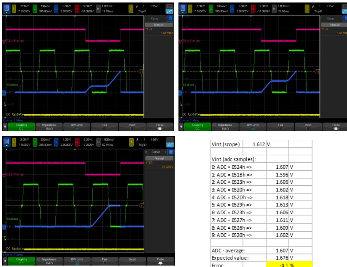
Figure 146. Example with all channels at 50.7% and gradual delay (2 nd , 3 rd and 5 th pulse)
