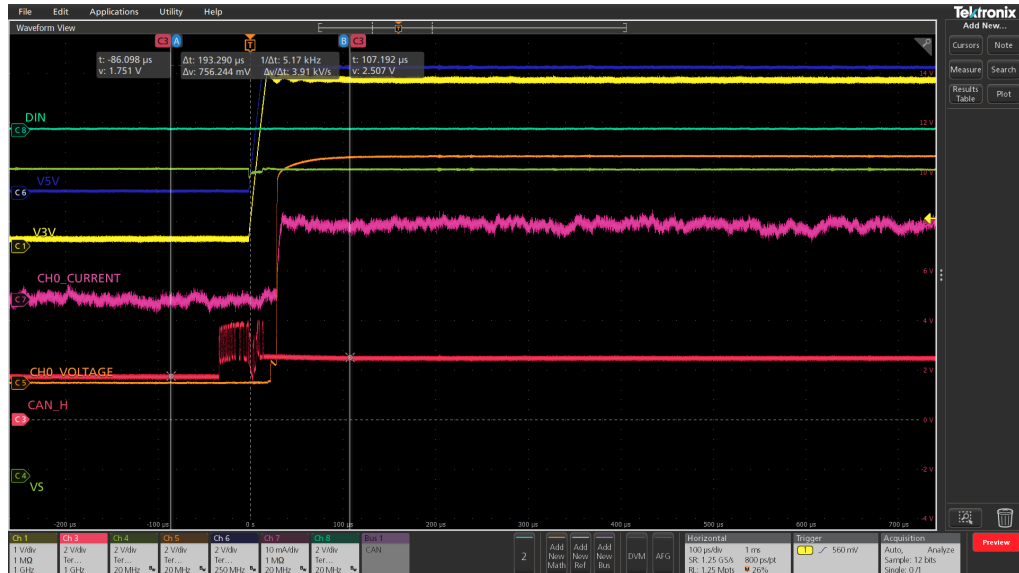
Figure 8. Device transition from stdby to Fail Safe after wakeup frame
