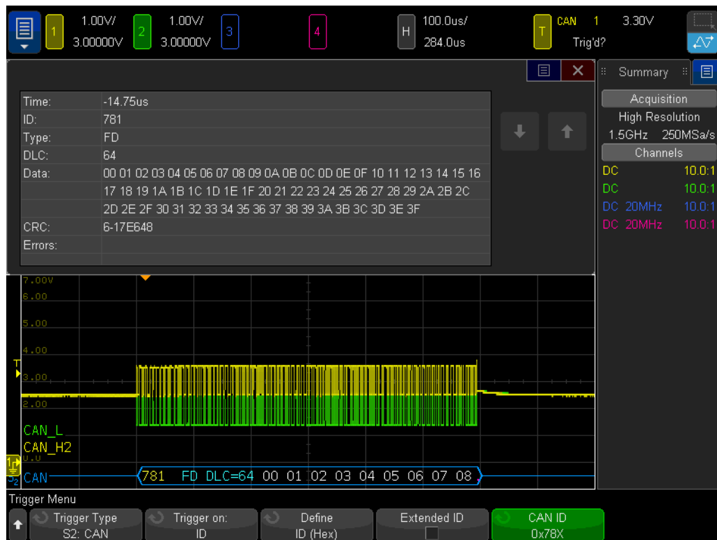
Figure 46. Broadcast PWM data send to ChainID=1 (test case 1)
