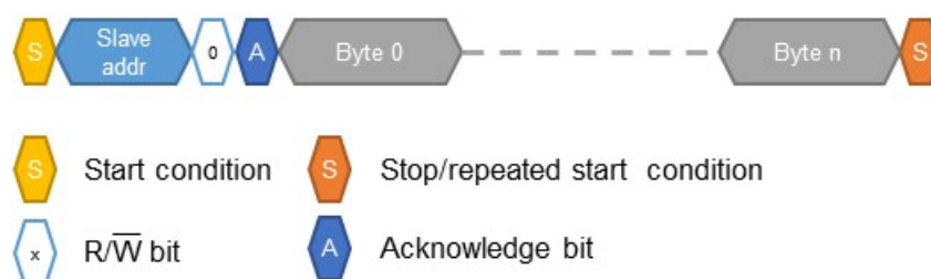
Figure 7. I 2 C Write operation description
