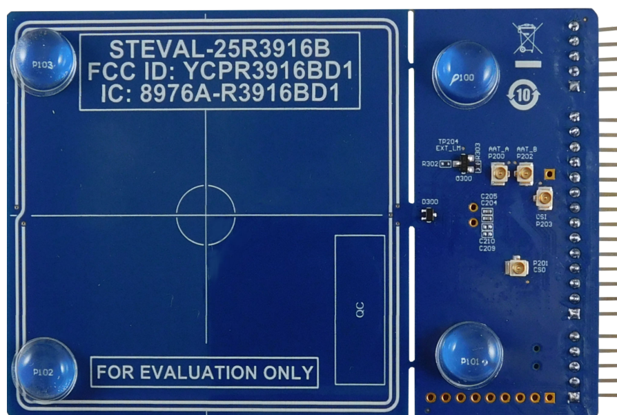
Figure 8. STEVAL-25R3916B expansion board layout (bottom view)
