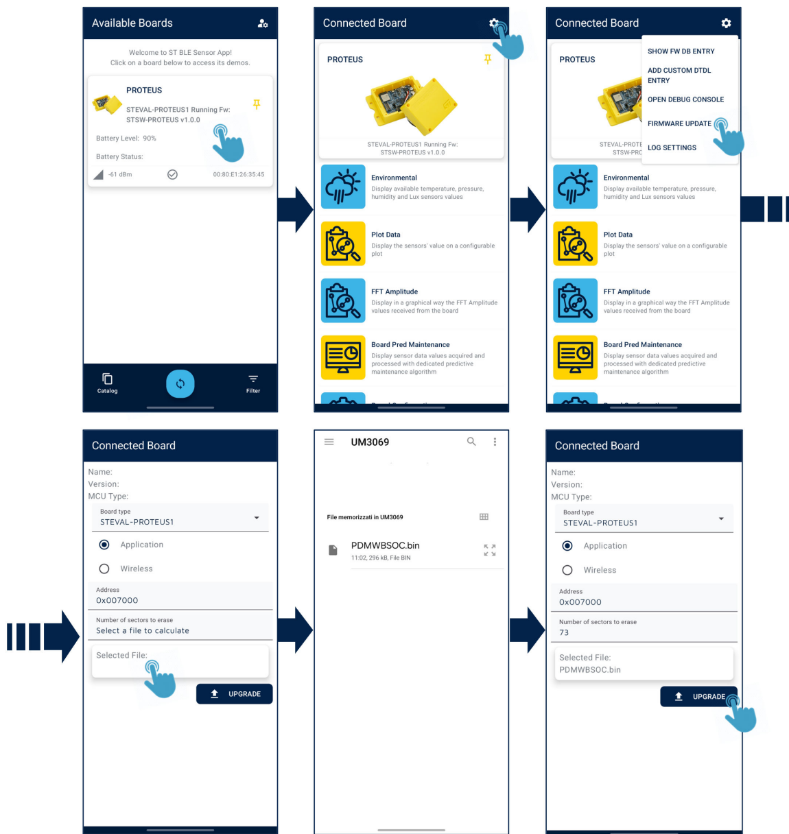
Figure 11. Start FUOTA and select FP-AI-PDMWBSOC binary application
