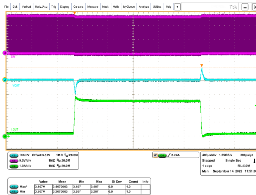
Figure 51. V_{IN} = 24\text{ V} ; V_{OUT} = 5\text{ V} ; I_{OUT\text{ MAX}} = 3.407\text{ A} ; I_{OUT\text{ MIN}} = 3.207\text{ A}
