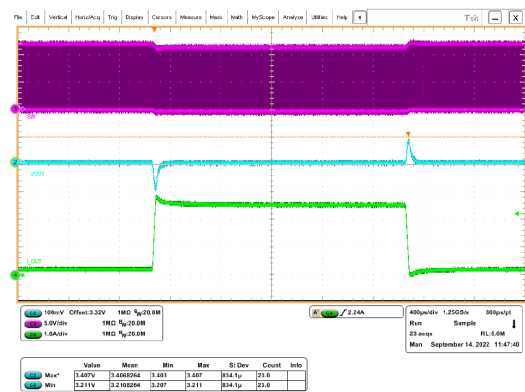
Figure 50. V_{IN} = 12\text{ V} ; V_{OUT} = 5\text{ V} ; I_{OUT\text{ MAX}} = 3.407\text{ A} ; I_{OUT\text{ MIN}} = 3.211\text{ A}
