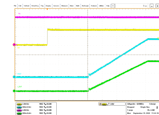
Figure 63. Power-up from EN: V_{IN} = 12\text{ V} ; V_{OUT} = 3.3\text{ V} ; I_{OUT} = 2\text{ A}
