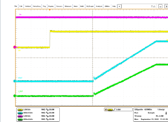
Figure 64. Power-up from EN: V_{IN} = 15.5\text{ V} ; V_{OUT} = 3.3\text{ V} ; I_{OUT} = 2\text{ A}
