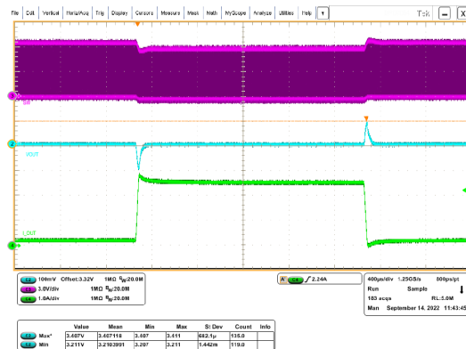
Figure 49. V_{IN} = 6.5\text{ V} ; V_{OUT} = 3.3\text{ V} ; I_{OUT\text{ MAX}} = 3.407\text{ A} ; I_{OUT\text{ MIN}} = 3.211\text{ A}
