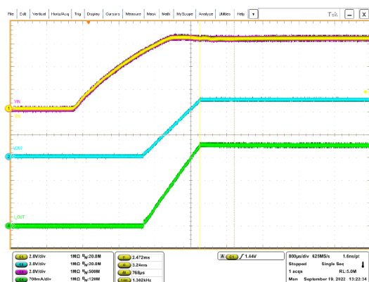
Figure 95. V_{IN} = 6.5\text{ V} ; V_{OUT} = 5\text{ V} ; I_{OUT} = 2.5\text{ A}
