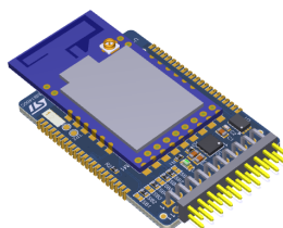
Figure 12. MB1400 Wi-Fi® module
