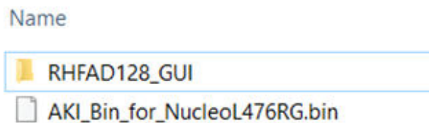
Figure 5. There are two documents: RHFAD128_GUI folder containing the RHFAD128_GUI.exe to launch on the laptop - AKI_Bin_for_NucleoL476RG.bin to upload in the Nucleo
